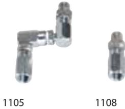
To handle grease hoses easily even at high pressure. For best results, use a straight swivel between the pump and distribution hose and a Z swivel between the hose and grease control gun. Maximum working pressure: 7000 psi (500 bar).
