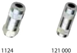
For use with air operated pumps or hand greasing units on hydraulic type nipples (DIN 71412). Connector head, contact surface and jaws manufactured in hardened steel. Maximum working pressure: 7000 psi (500 bar). Connection thread: 1/8" NPTF.
