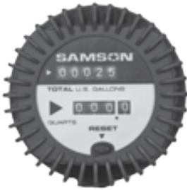
Oval gear meter with mechanical, odometer style display for use with lubricants up to SAE 140. Partial reading up to 999.9 quarts and non-resettable totalizer registers in gallons. Meters are factory calibrated for maximum accuracy and include protective rubber shroud.
