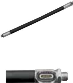
Double steel braid safety rubber hoses for use with air operated greasing equipment. Maximum working pressure: 7000 psi (500 bar). 1/8" NPTM threads.
