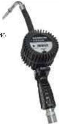
Oval gear meter with mechanical, odometer style display for use with lubricants up to SAE 140. Partial reading up to 999.9 quarts and non-resettable totalizer registers in gallons. Meters are factory calibrated for maximum accuracy and include protective rubber shroud. The meter is flange coupled to a durable but lightweight oil control gun that incorporates a rugged ball bearing inlet swivel with filter.
