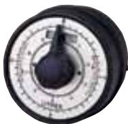
Oscillating piston design for rugged dependability; for use with SAE 5 to 140 oils or glycol solutions. 1/2" NPTF inlet/outlet, 1000 psi max.
